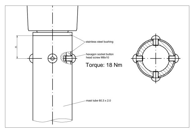
NOTE: For mounting in mast tubes with inner diameter 55.0 mm the two grey plastic adjusting rings have to be removed from the stainless-steel bushing before insertion.
