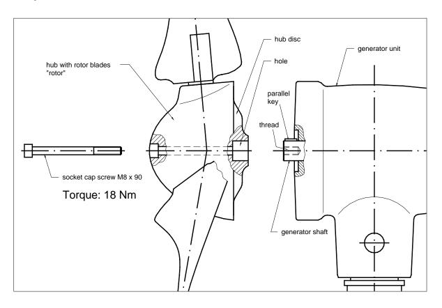
NOTE: To avoid damage inside the generator do not push the generator shaft into the generator housing (loss of warranty!).
