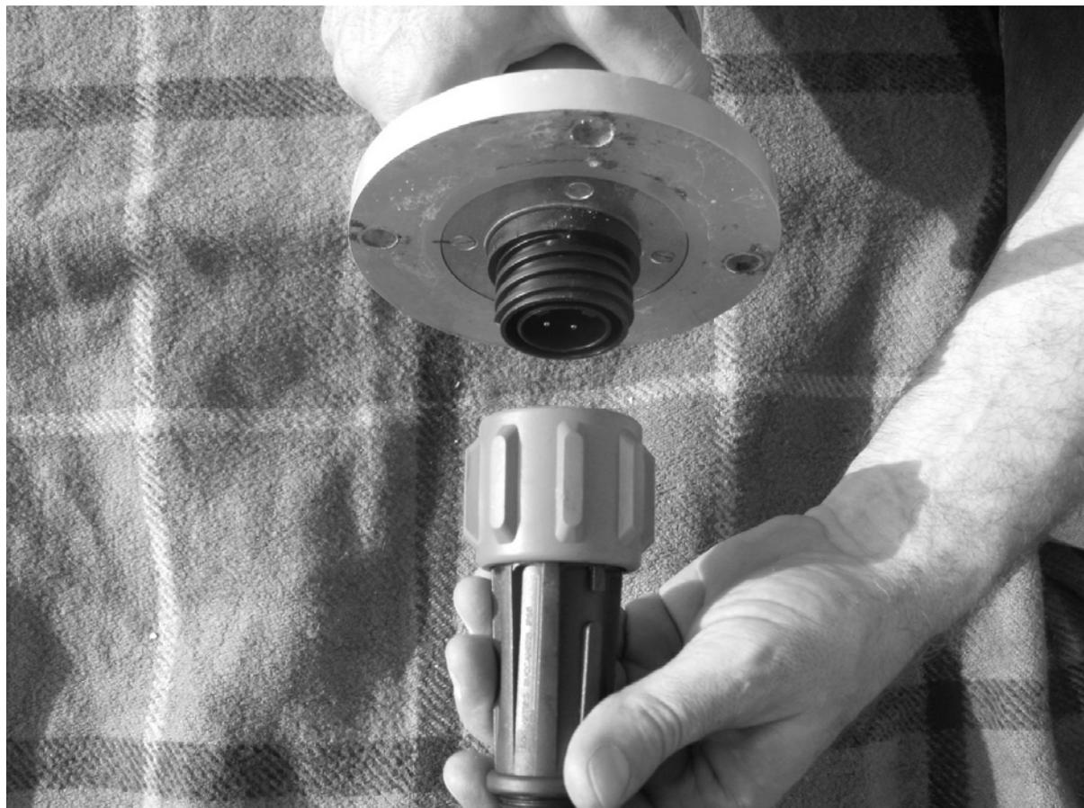
Move the generator unit carefully towards the mast flange.
