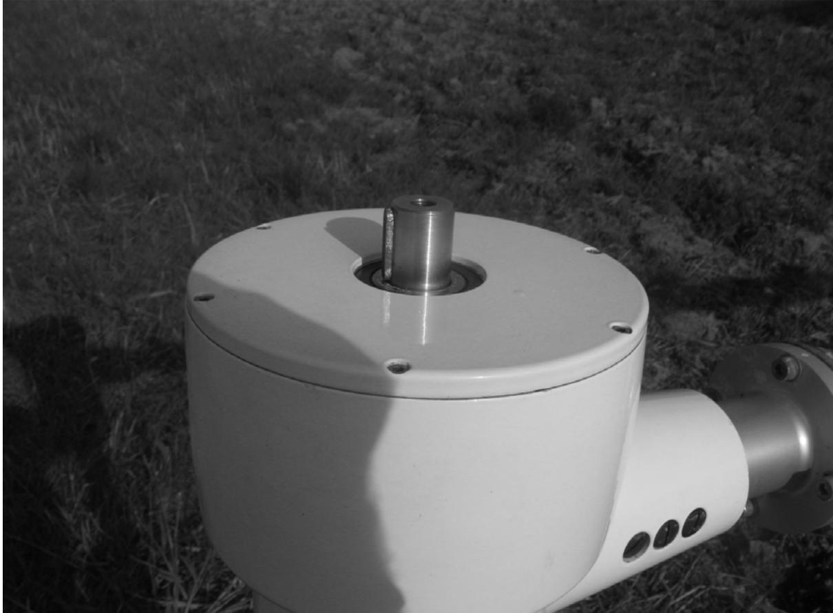
Align the hub and carefully slide onto the generator shaft.
