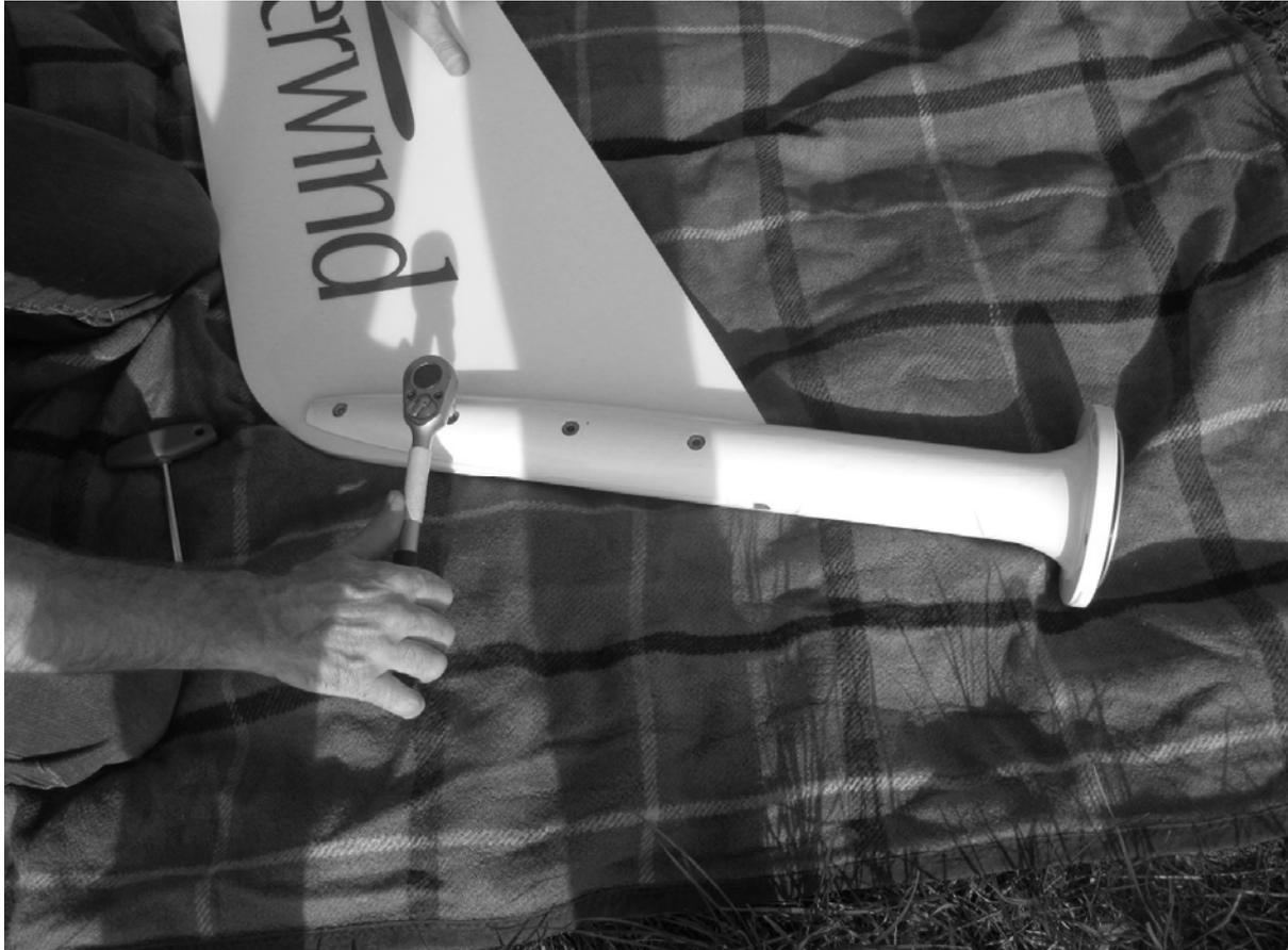
**WARNING:** Remember that many of the wind turbine components are made of high quality aluminium as well as stainless steel. Damage may result if torque specifications are ignored!
