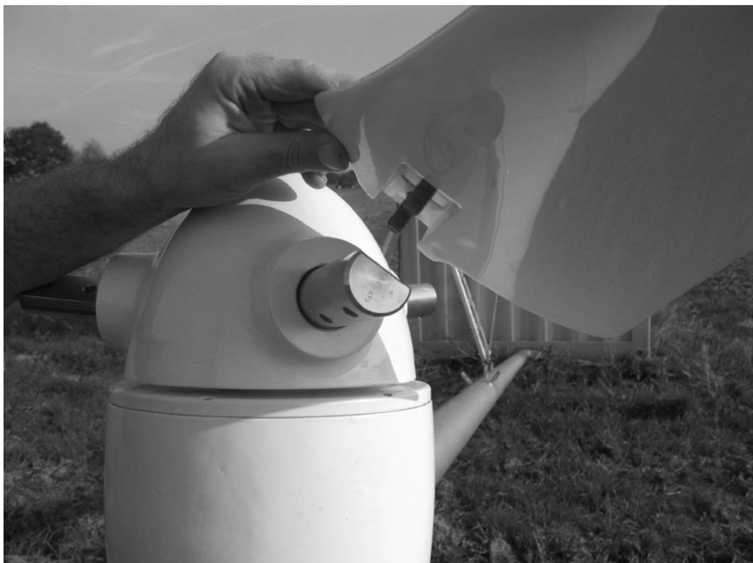
Feed both screws a few millimetres into the threads of the axle, then slide the rotor blade towards the axle.
