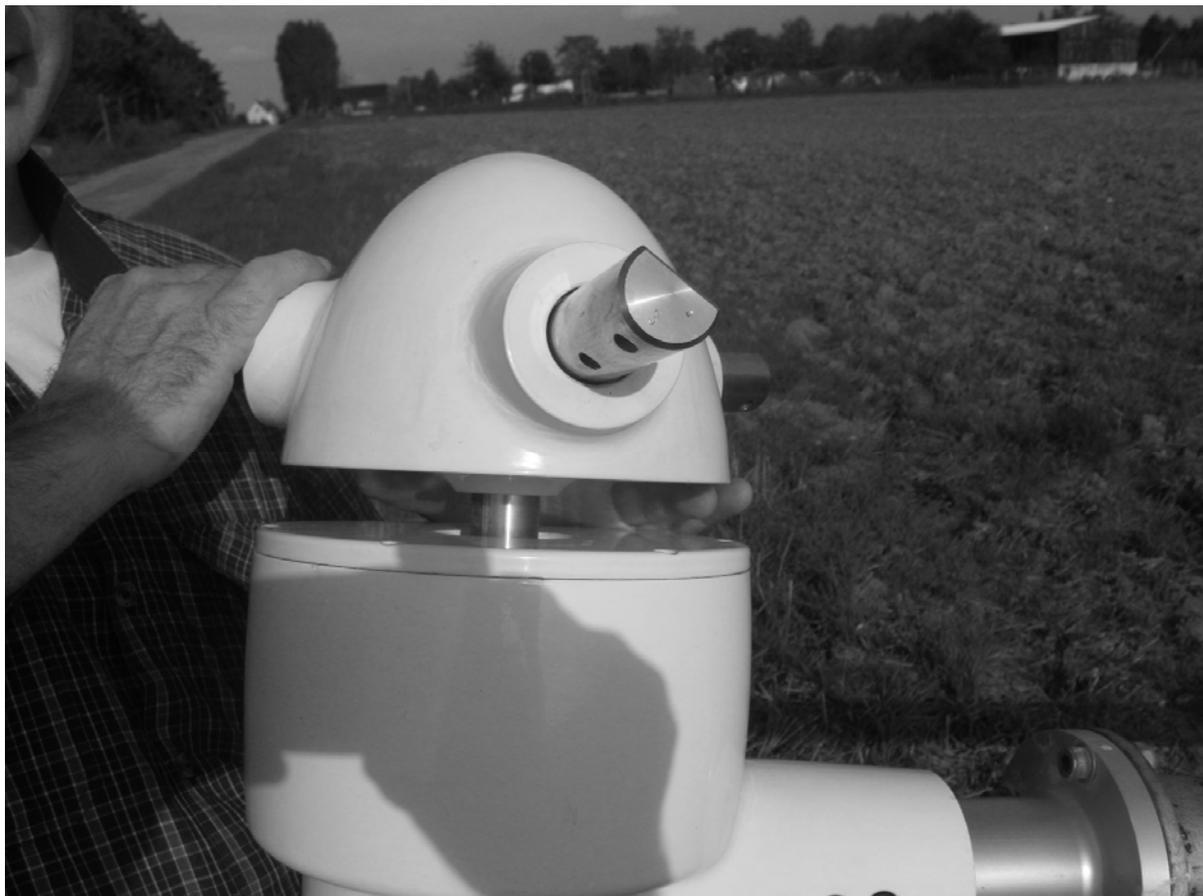
**NOTE:** When sliding the hub onto the generator shaft ensure the parallel key slides into the corresponding keyway (groove) of the hub.
