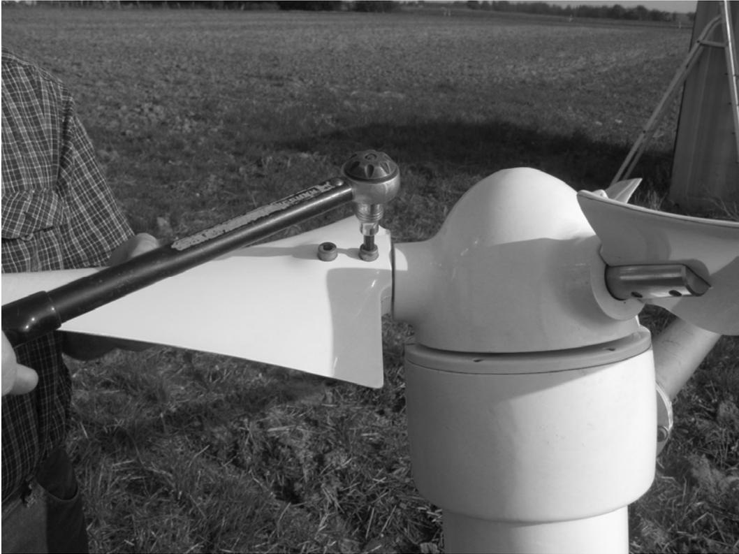
**NOTE:**           Ensure each axle is correctly inserted into the recess of its respective blade.
