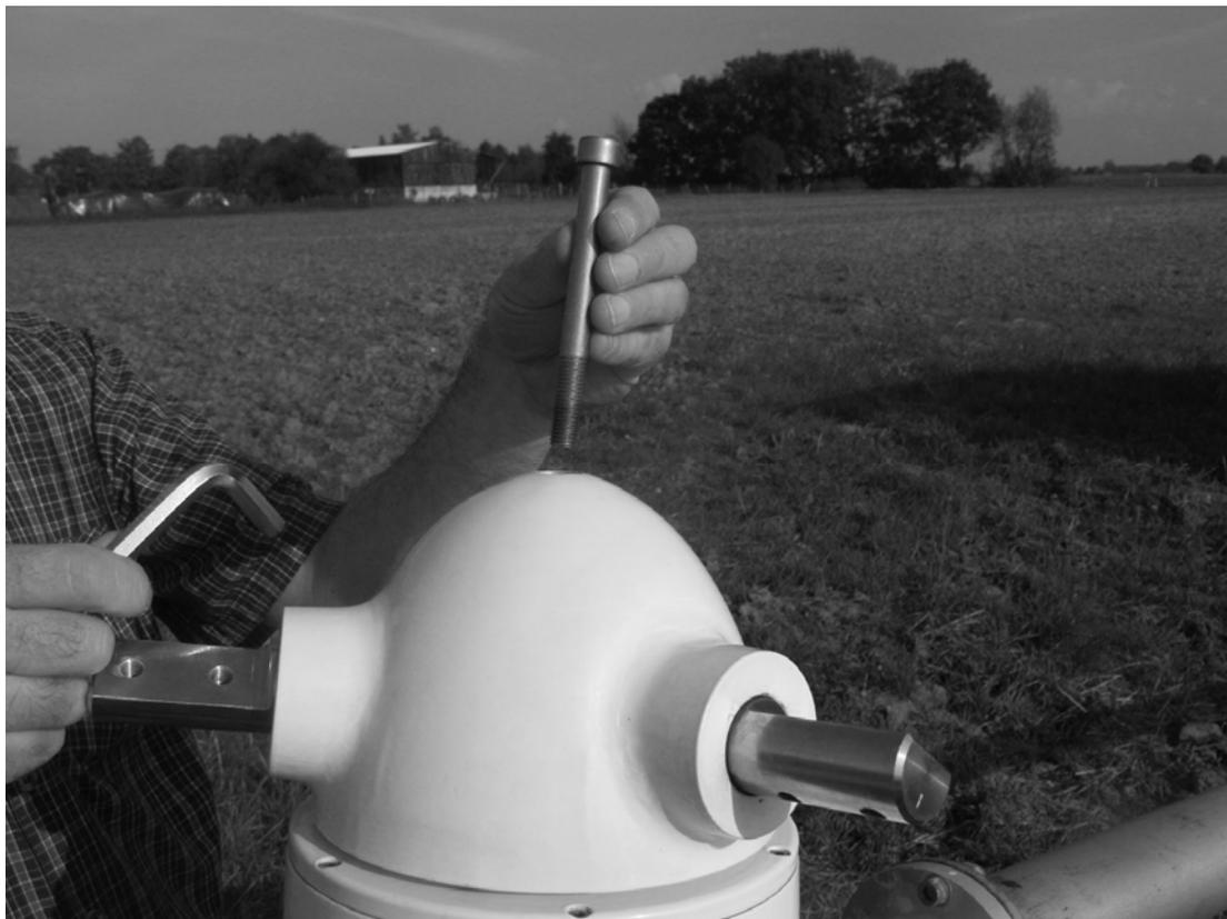
Tighten and torque the screw to 50 Nm (SAE 36.9 foot-pounds).
